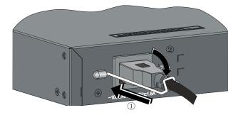
Figure 3-17 Connect an AC power cord to a vertical AC power socket (1)
